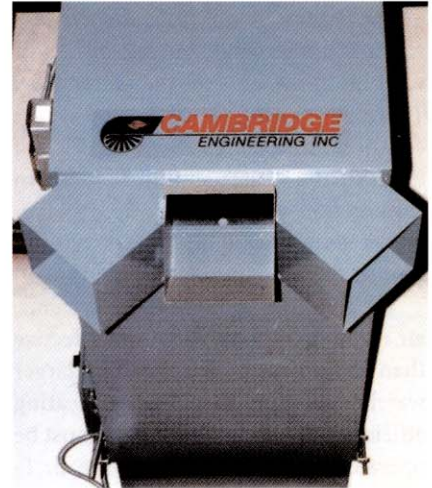
A direct-fired gas space heater installed through the wall near the ceiling is constructed of a gas burner and blower. This arrangement delivers high levels of heat using a minimal amount of air from outside the warehouse.
